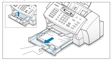
2. Remove the jammed paper by carefully pulling it out of the tray.
